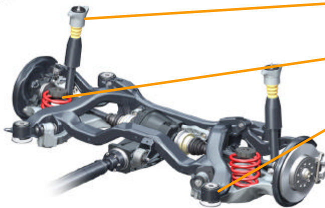
Audi A4 quattro Spurgesteuerte Trapezlenker-Hinterachse Self-tracking trapezoidal-link rear axle 9304
